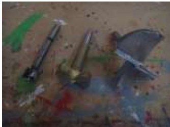
These are the forstner bits we have in school. 18, 38, 50 and 60mm
