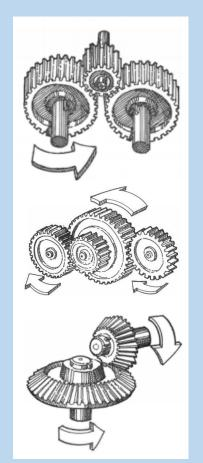
**This is a simple gear train -** This is when a number of gears are connected together in a train.
