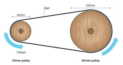
4) Calculate the output speed of the pulley system and show your working. (3)
